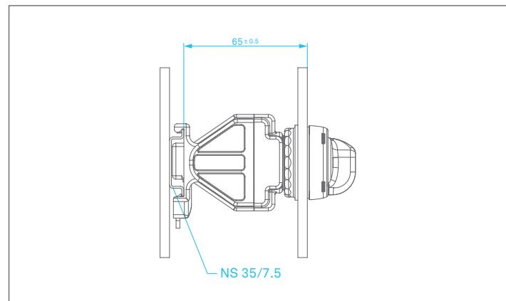
Front mounting is only possible for Control switch module with position selector switches with protective collar.
