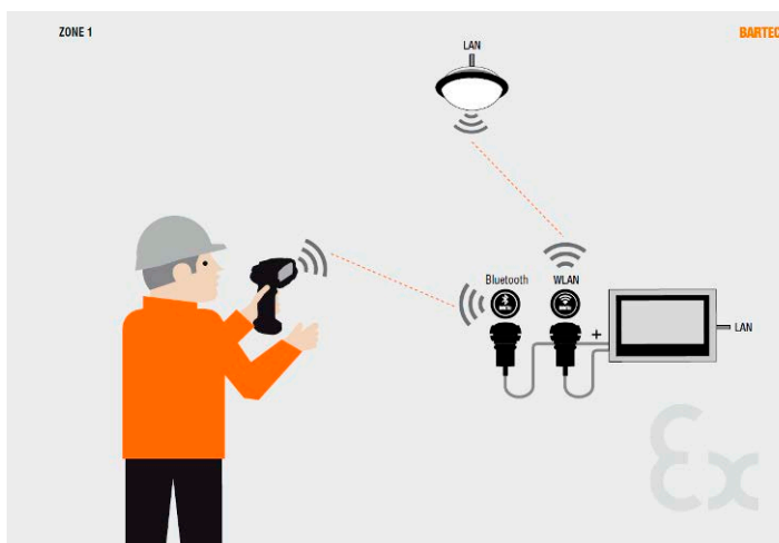
HMI system in Zone 1 with Bluetooth scanner series BCS3678-IS (Zone1) and connection to the network via Wireless X AP.
