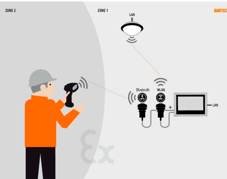
HMI system in Zone 1 with Bluetooth scanner series BCS3678-NI (Zone 2) and connection to the network via Wireless X AP
